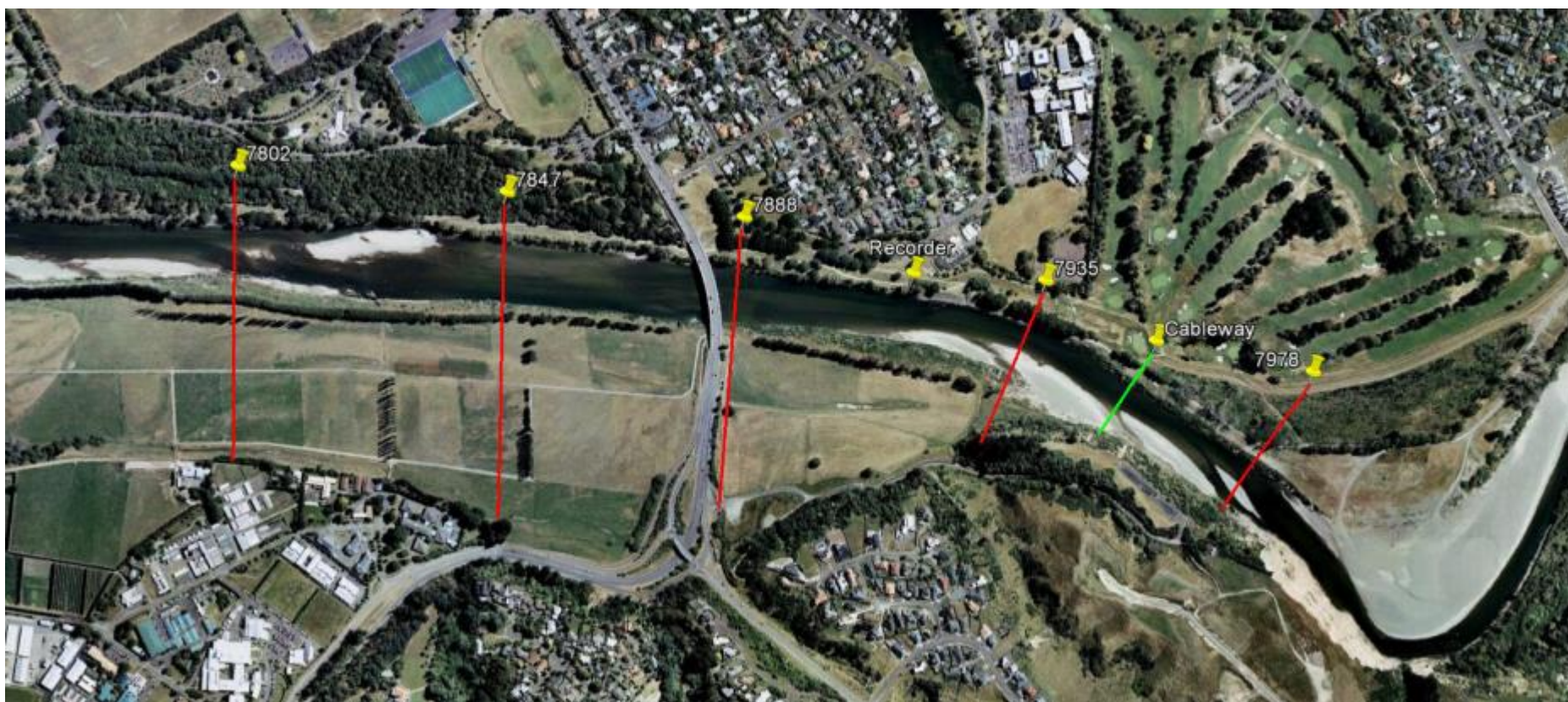
Figure 18 – Recording reach at Manawatu at Teachers College showing location of recorder tower, gauging cableway and surveyed river cross-sections
