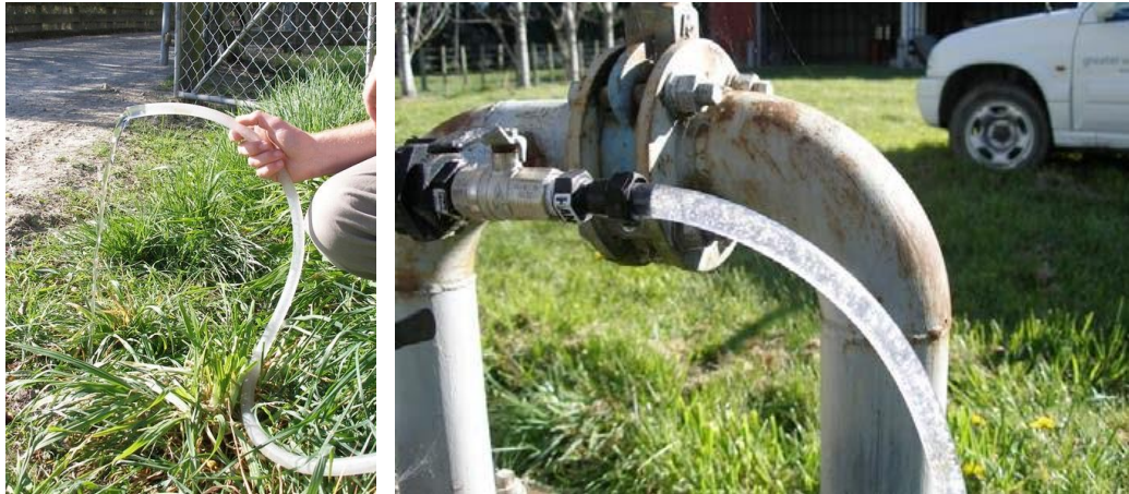
Figure 3 – A suitable pump rate will ensure laminar flow from the outlet point (left); aerated flow (right) is not appropriate
