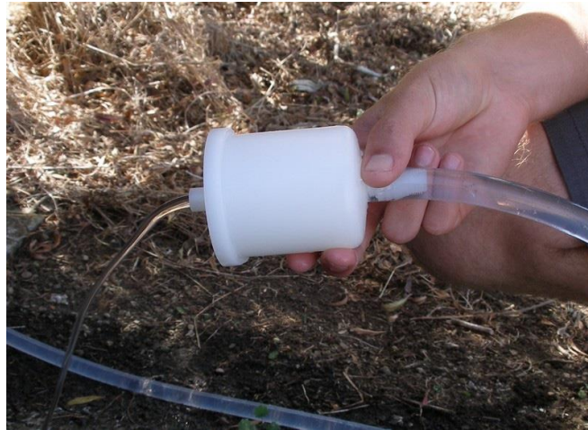
Figure 9 – An in-line filter attached to the sample point using clean tubing
