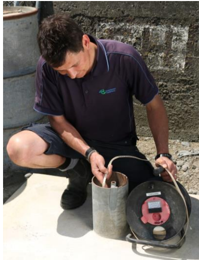
Figure 1 – Water level in non-artesian conditions can be measured using a dip tape and the depth recorded relative to a known point on the well
