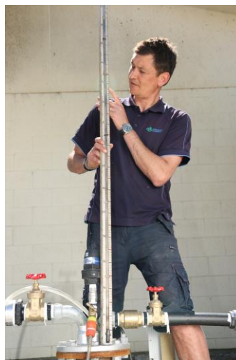
Figure 2 – Artesian head can be measured using a clear tube and a staff gauge
