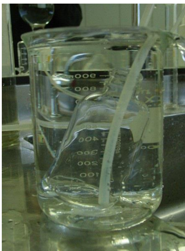
Figure 7 – Collection of a water sample in isolation from the air
