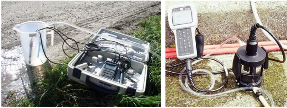
Figure 4 – Water from the pump outlet can be passed through an open container (left) or a flow cell (right)
