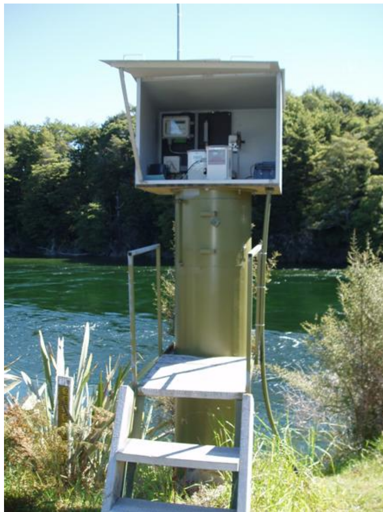
Figure 13 – Typical stilling well housing design.
