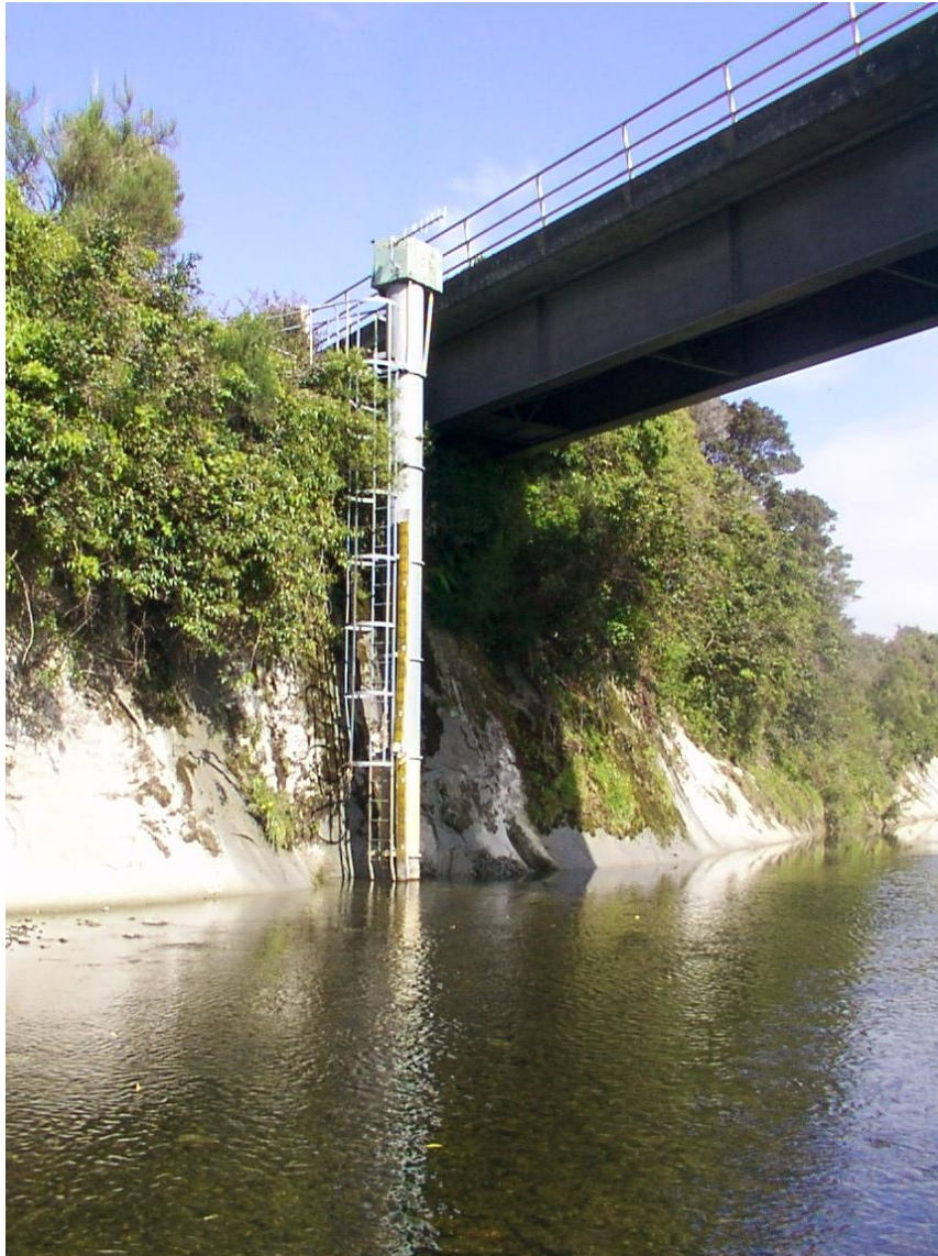
Figure 10 – Stilling well with multiple sections and housing.
