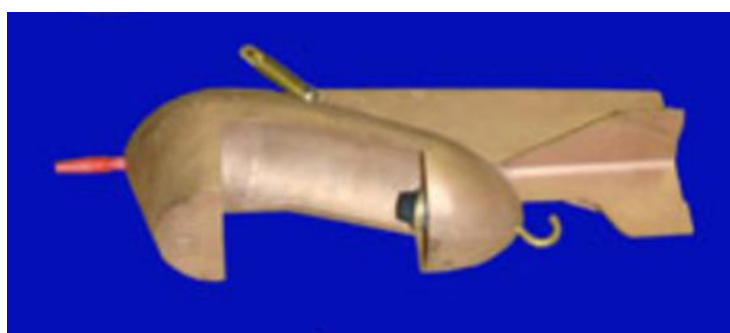
Figure 4-3 – DH-76 handline-suspended depth-integrating sampler.
