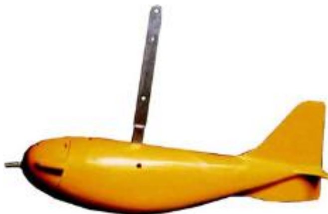
Figure 4-4 – D-74 cable-and-reel depth-integrating sampler.
