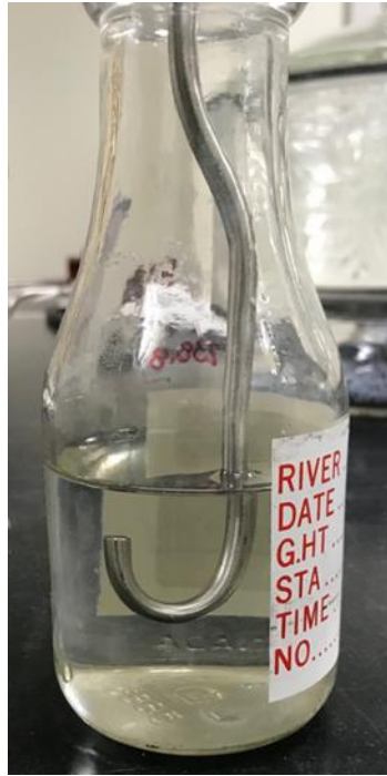
Figure 11-1 – J-tube (shown inside a glass sample bottle), used for decanting surplus clear water from a settled sample prior to evaporation when using ASTM D3977-97 (2019) Method A for SSC analysis. Photo courtesy of Stephen Low, USGS.
