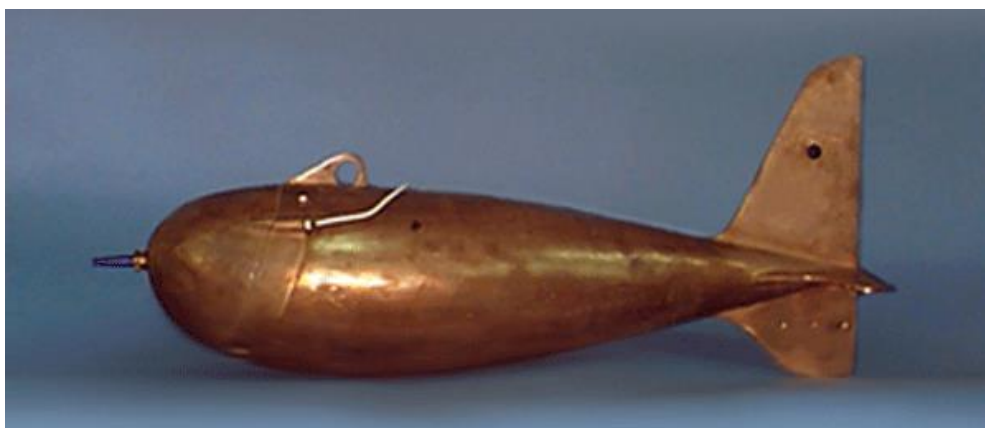
Figure 4-6 – P-61 cable-and-reel point sampler.
