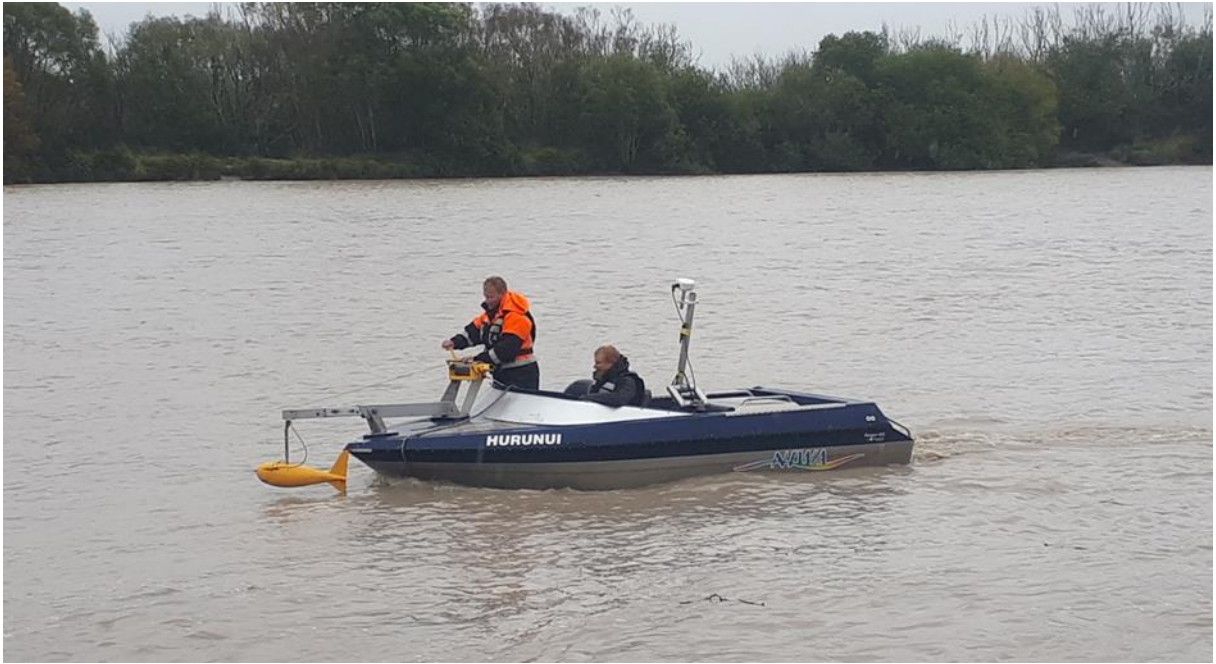
Figure 2-1 – A 48-kg US P-61 point sampler deployed from a jet-boat using a bow-boom and gauging reel. Note GPS antenna to assist navigation across the sampling section.
