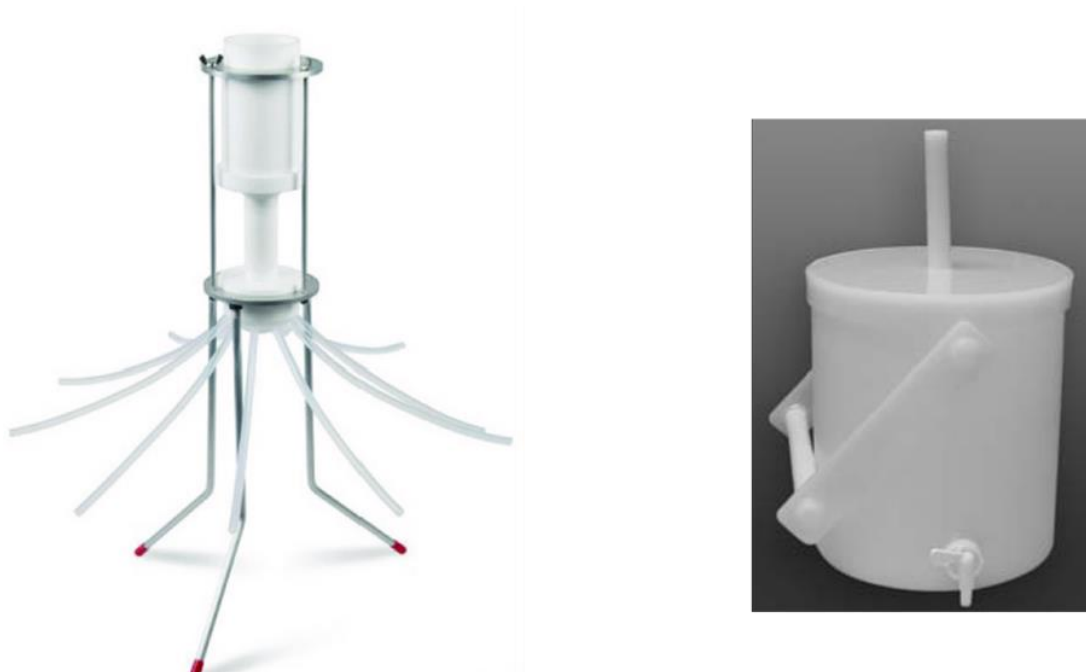
Figure 12-1 – Sample splitters for reducing sediment mass for particle size analysis. Left: cone splitter (the original sample drains into multiple outlet pipes). Right: churn splitter (a sub-sample is drawn off via the spigot while the piston agitates and mixes the original sample).
