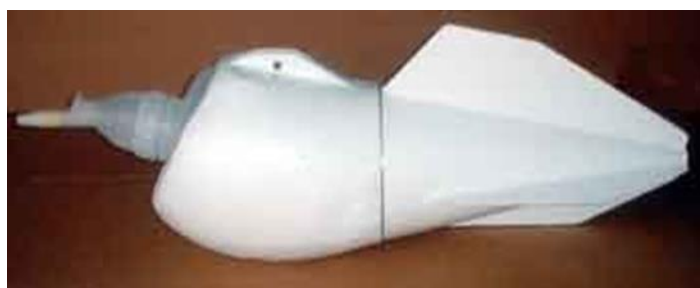
Figure 4-5 – D-77 cable-and-reel depth-integrating sampler.
