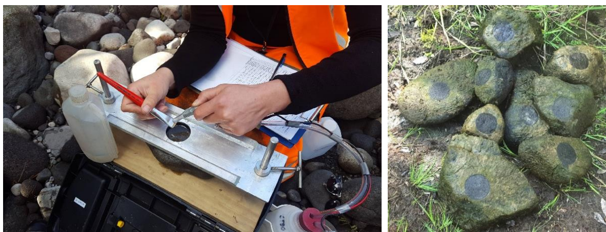
Figure 11: A vacuum pump system (left) and rocks from which periphyton has been removed
