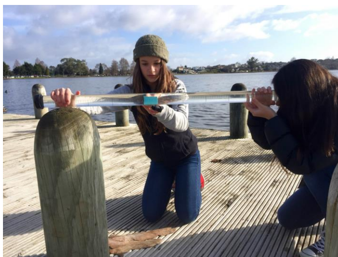
Figure 8 – Measuring visual clarity through a tube
