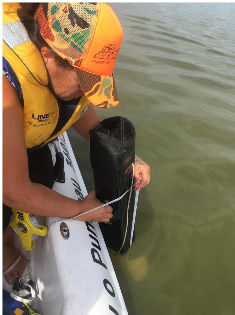
Figure 6 – Measuring visual clarity from a boat with a Secchi disk
