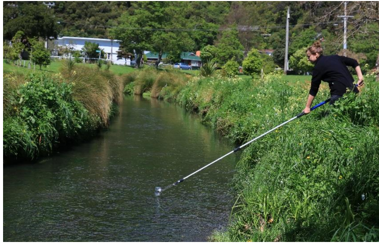
Figure 11 – Water sample collection using a telescopic pole
