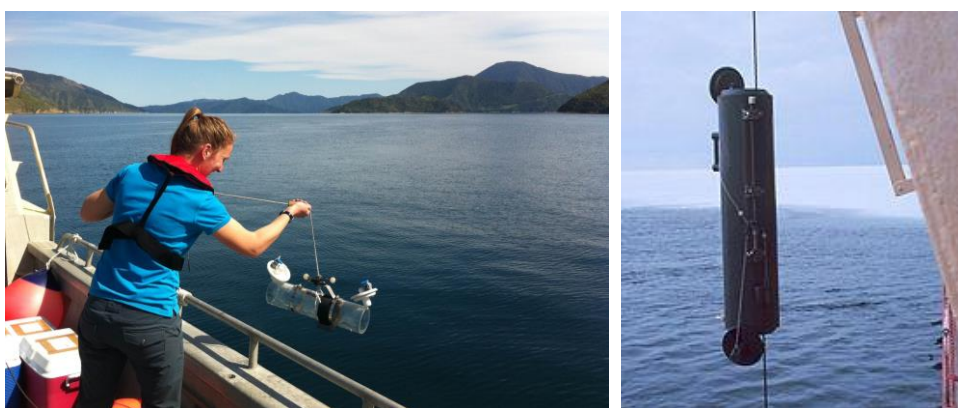
Figure 12 – Deploying Van Dorn (horizontal, left) and Niskin (vertical) water sampling devices
