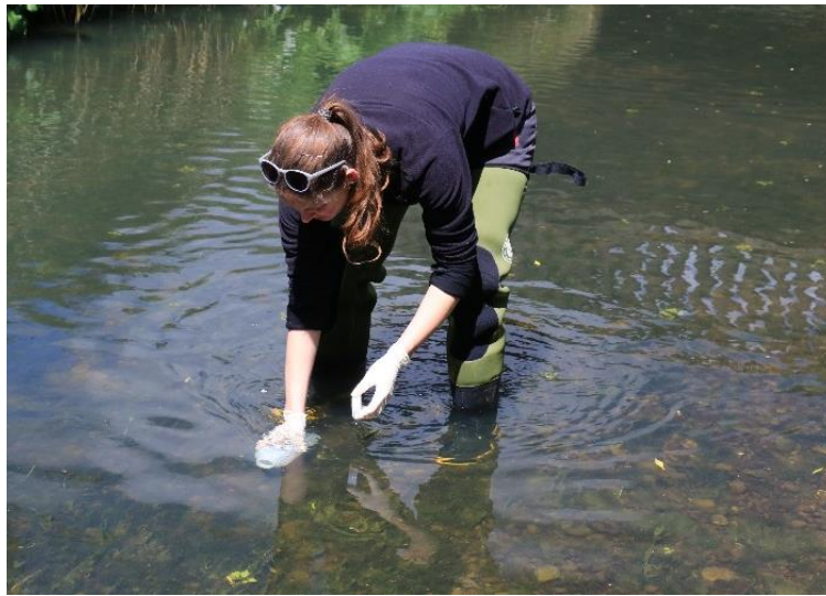
Figure 10 – Wading and water sample collection by hand
