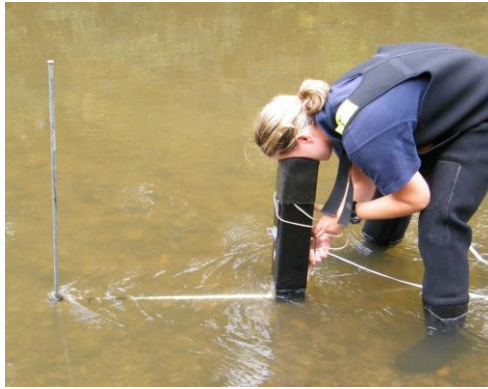
Figure 5 – Using a periscope viewer to make black disk observations
