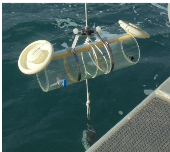
Figure 4. Set Van Dorn bottle being lowered into the water.
