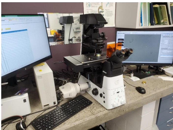
Figure 2: An inverted microscope with counting chamber.
