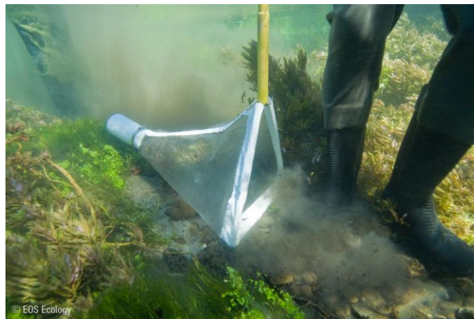
Figure 8 – Kick-net sampling in a hard-bottomed stream
