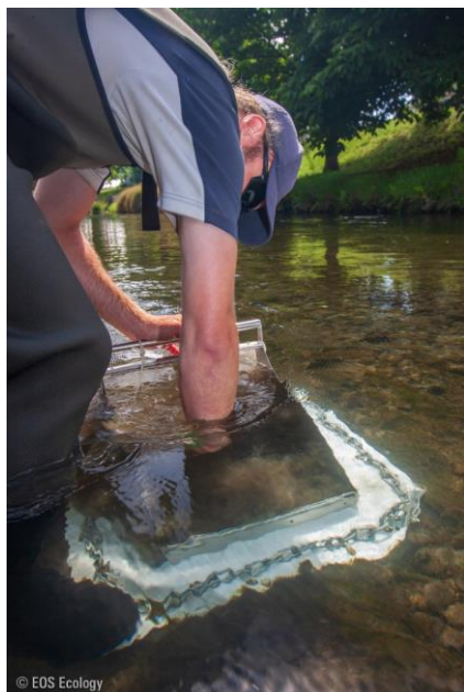
Figure 10 – Using a Surber sampler in shallow hard-bottomed streams – note the use of a heavy chain to form an effective seal between the base of sampler frame and the streambed (left)
