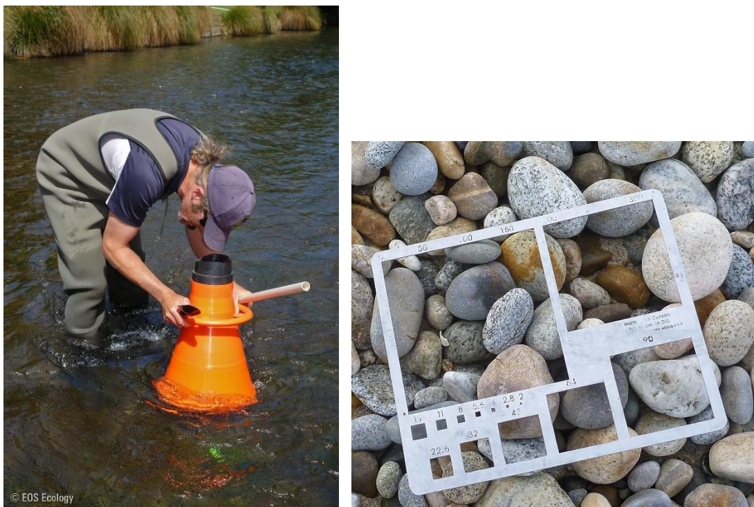
Figure 14 – Assessing streambed substrate cover using an underwater viewer (left) and substrate size using a gravelometer (right)
