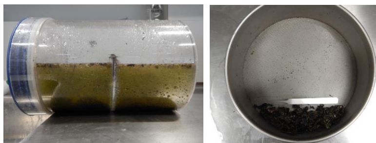
Figure E1 – Barrel splitter (left) and split sample contents captured in a sieve
