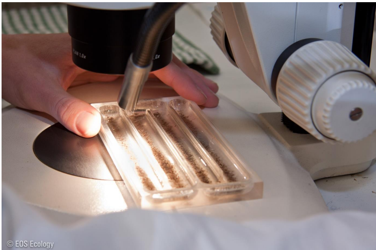
Figure 17 – Identification of macroinvertebrates in a subsample under a binocular (dissecting) microscope with additional lighting Photo: EOS Ecology
