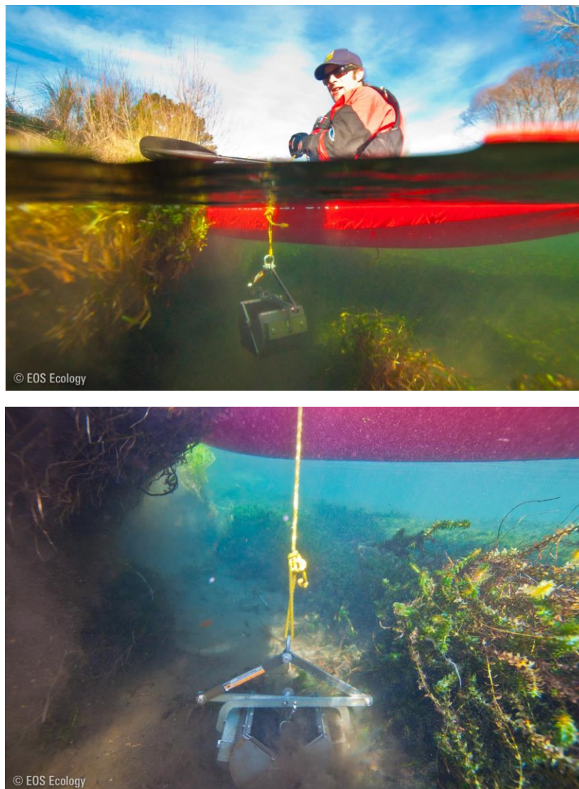
Figure 11 – Sampling a non-wadeable stream from a kayak (top) using a Polman grab sampler
