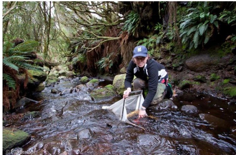
Figure 10 – Using a Surber sampler in shallow hard-bottomed streams – note the use of a heavy chain to form an effective seal between the base of sampler frame and the streambed (left)
