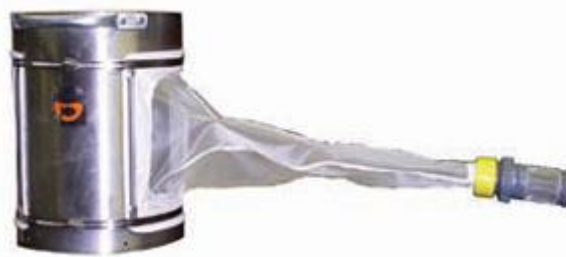
Figure 3– A Hess sampler with capacity to attach a sample container to the end of the net
